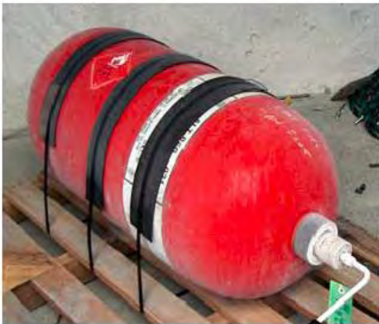
Figure 2. High Pressure Hydrogen storage tank [6]
