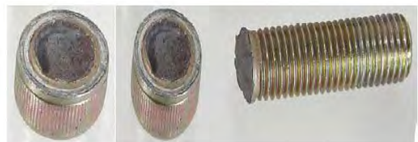
Figure 1. Typical Fastener Failure by Hydrogen Embrittlement [8]
